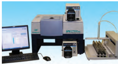
This spectrometer from Spectro Scientific uses FTIR spectroscopy to monitor in-service oil.
