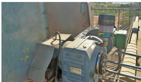
Figure 6. An exposed gearbox with a desiccant breather installed
