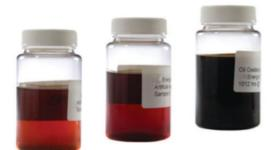
Any of these warning signs generally indicate that your oil has undergone a chemical change, and may no longer perform to its designed specifications. Premature breakdown of oil can be caused by a wide variety of conditions, including thermal stress, high pressure, fuel or gas entrainment, oxidation, and water contamination.
