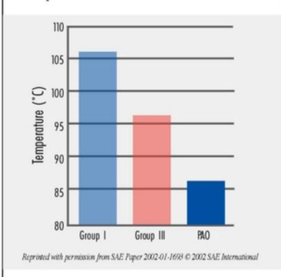
This lower operating temperature, along with the superior oxidative stability of PAO-based lubes can aid in increasing the service life of the lubricant and decrease the generation of corrosive agents that can damage your lubricated system.
