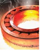
film keeping gears, bearings or slides apart is no longer present to support or protect the surfaces, surface-to-surface contact will occur. When two surfaces slide or rub together, friction is produced, and from friction comes heat. Check out this article on the ML site to discover the other signs that can indicate your machine is suffering from lubricant starvation as well as the most effective way to combat this condition.
