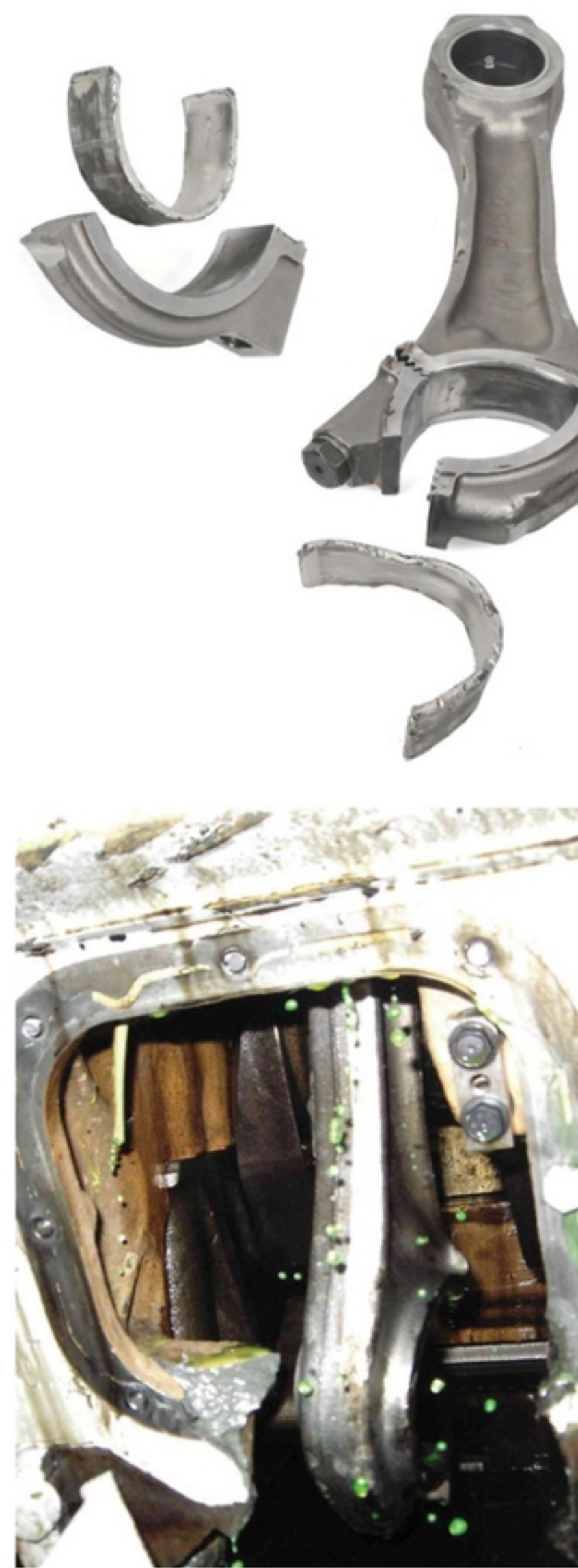
German naval ships suffered engine failures caused by connecting rods breaking off crank pins. Above bottom, an intact connecting rod. Above top, pieces from a broken conrod.
