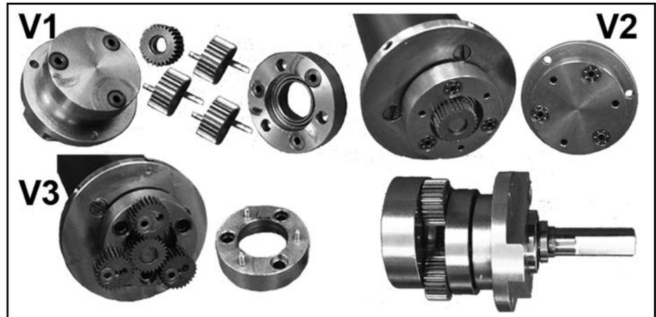
Figure 3 Versions 1, 2 & 3 Orbitless prototype gear-head.
