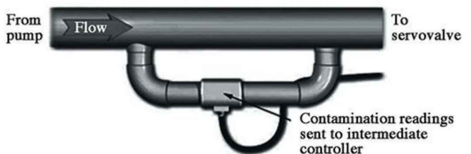
2. An online oil contamination sensor sends readings to an intermediate controller that signals the filter to operate when contamination levels exceed desired standards.
