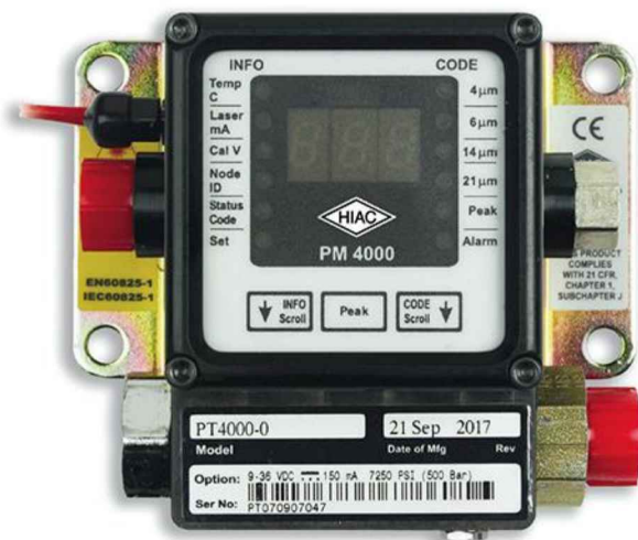
5. In this online particle counter, when a particle passes through a laser beam that lands on photodiodes, it reduces the amount of light received by the diodes and determines the size of the particle.
