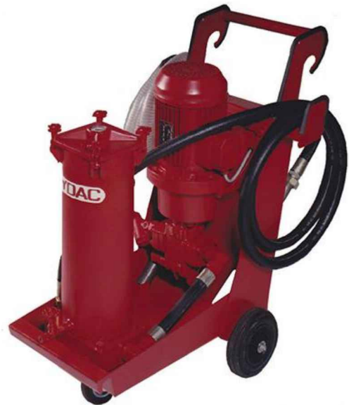
6. In one 20-minute filtration cycle, the system's mobile filtration unit can filter all 2,000 l of oil in the HMO tank.
