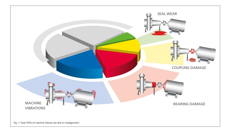
When a machine vibrates, its skids can move and affect its alignment. When minor process parameters such as pressure or temperature are modified, alignment can change. Even the simple and natural succession of the seasons can alter alignment and put machine assets at risk. Effectively countering the factors that
