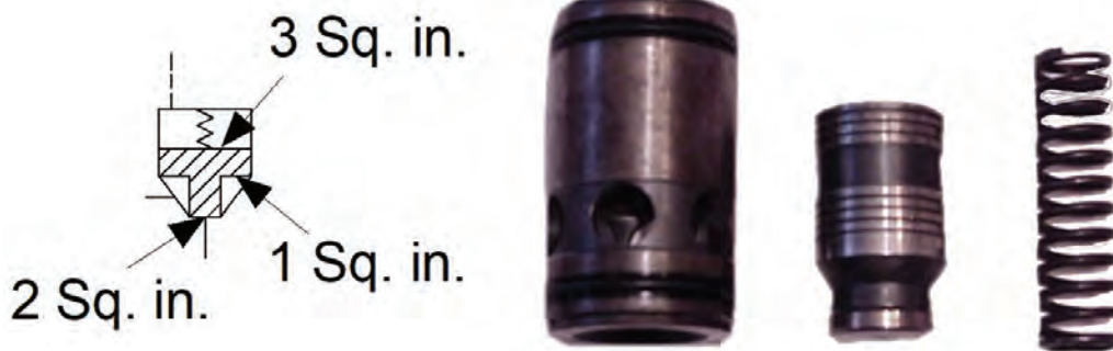
Figure 1. A schematic symbol for a logic valve alongside the valve it represents
