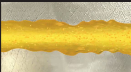
Figure 2 | The metal surfaces move closer together in the mixed film lubrication regime where industrial gear oils (lubricant film is shown in orange) also operate.
