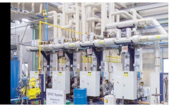
The new highly efficient lube oil blending plant designed and successfully started up by ABB in China for a global energy and petrochemicals group is able to face the rising demand for large and bulk orders. It incorporates In-Line Blending technology and Lubcel™ control system to facilitate the fast and accurate simultaneous blending of large volumes of lubricants and guarantee on-time deliveries of on-spec products. www.abb.com/industries
