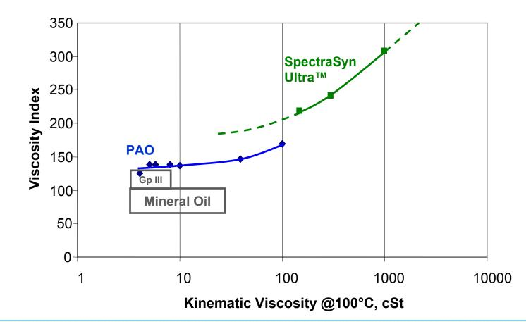
At equivalent viscosity, SpectraSyn Ultra<sup>™</sup> is 40 VI higher than high viscosity PAO, enabling formulations with better protection at high temperatures and reduced energy losses and easier starting at low temperatures
