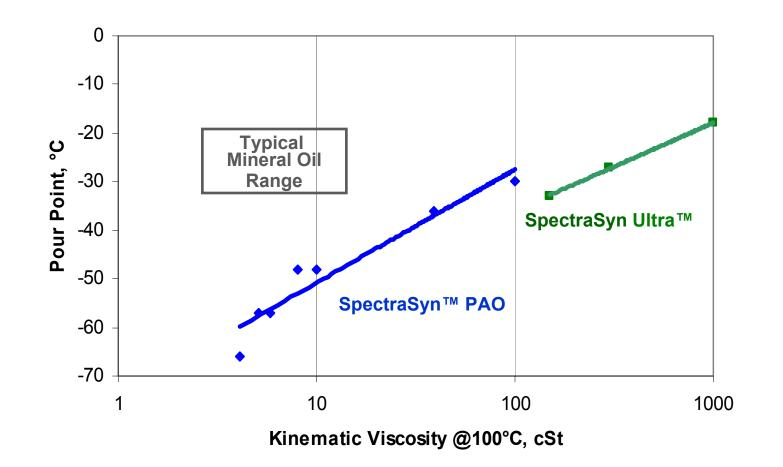
Spectrasyn<sup>™</sup> PAOs flow easily at low temperatures.
