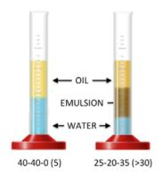
graduated cylinder. The test is concluded after 30 minutes or when the oil and water separate to an acceptable level, whichever comes first.
