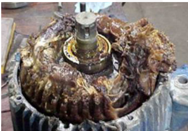
Figure 13: Failure Caused by Over Greasing of Motor
