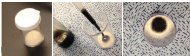
Figure 3: FDM sample vial and dispensing the oil sample onto the felt disc using a graduated disposable pipette.
