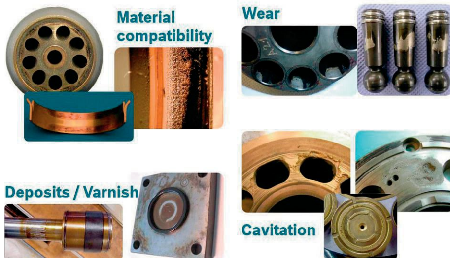
Figure 3. Causes of failure due to fluid
