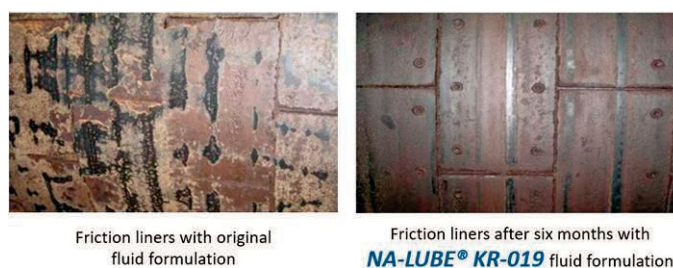
Figure 11. Continuous Hot Press Friction Liners after First Fluid Change Interval
