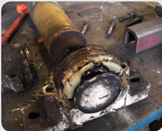
Figure 12 & 13: Housing overfilled. No grease drainage.
