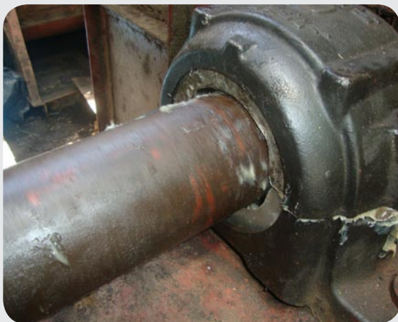
Figure 7 & 8: Home made seal from an aluminum sheet. Note the gap between "seal" and shaft.
