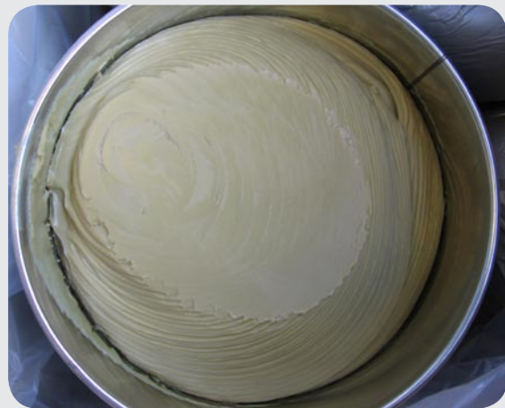
Figure 2: Grease stored for long time (Grease hardening)
