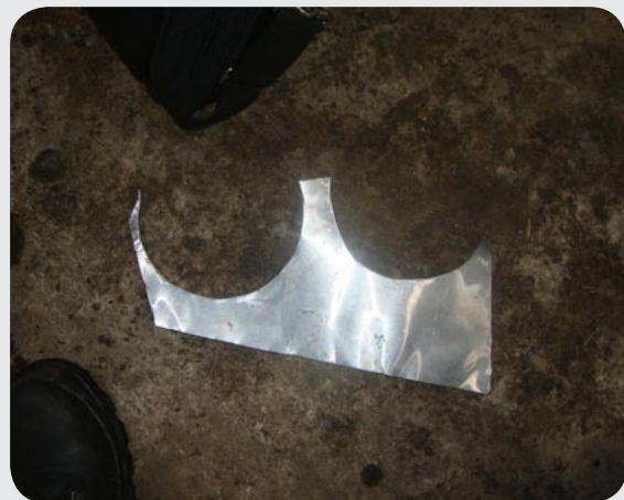
Figure 7 & 8: Home made seal from an aluminum sheet. Note the gap between "seal" and shaft.
