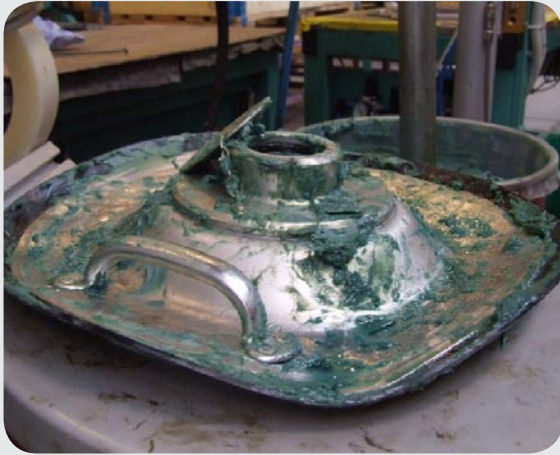
Figure 3: Dirty grease pump follower plate.
