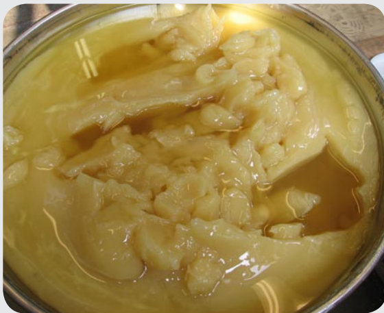
Figure 1: Grease stored for long time (Excessive oil separation)
