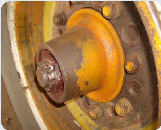
Figure 5 & 6: Grease cap lost and contamination ingress leading to bearing failure.
