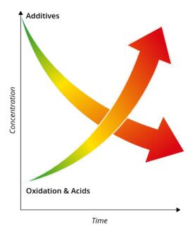
The rate of oil degradation and additive depletion will vary tremendously depending on several controllable factors.
