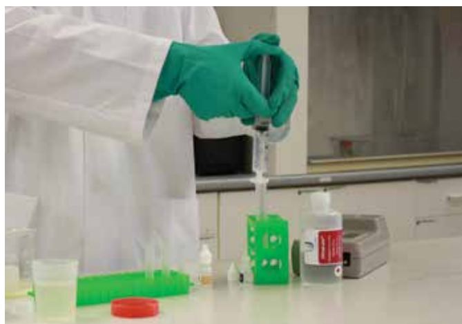
Figure 5 | A new ATP test has just been approved by ASTM to measure the microbe population density in a MWF system. (Courtesy of LuminUltra™ Technologies Ltd.)
