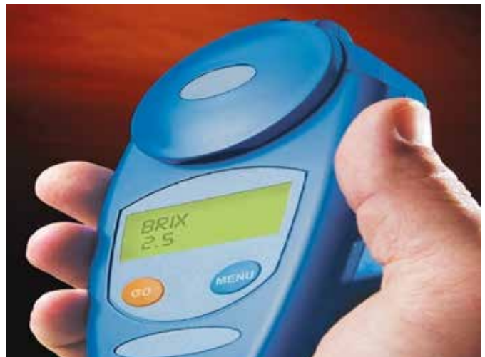
Figure 2 | Digital refractometers are better able to handle the measurement of MWFs under more adverse conditions. They also provide better accuracy and precision than analog refractometers. (Courtesy of MISCO Refractometers)
