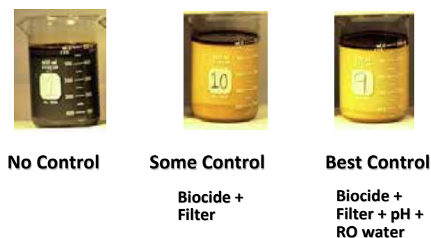
Figure 1 | Three samples from a series of 15; 20 weeks after having been diluted to end-strength (5 percent v/v). Sample 1 was prepared using tap water, but contained no microbicide. Sample 10 was treated with a microbicide and was filtered periodically. Sample 9 was similar to sample 10 except that it was diluted with high-quality (reverse osmosis) water and its pH was maintained at 9.2. Among the 15 samples only those that contained microbicide retained appearances similar to those of samples 9 and 10. The other 12 samples appeared similar to sample 1 at the end of 20 weeks. (Courtesy of STLE member John Burke)
