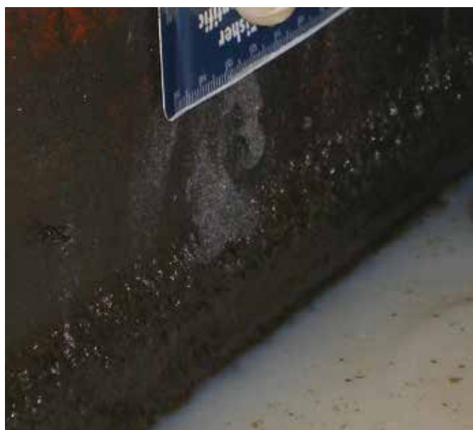
Figure 4 | Microbes can cause problems in MWFs systems by forming biofilms such as the one found here on the wall of a sump just above the MWF surface. (Courtesy of BCA Inc.)
