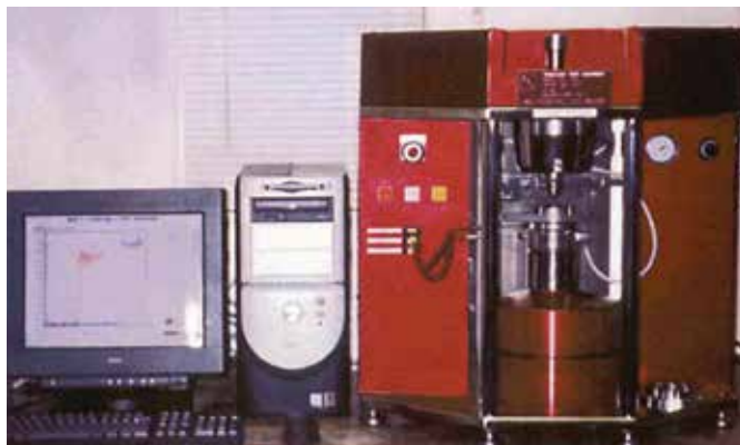
Figure 3 | The Multi Four-Ball Test Machine incorporates both the four-ball EP and wear testers into one computer-operated instrument to measure the extreme-pressure and wear properties of a MWF. (Courtesy of Engineered Lubricants Co.)
