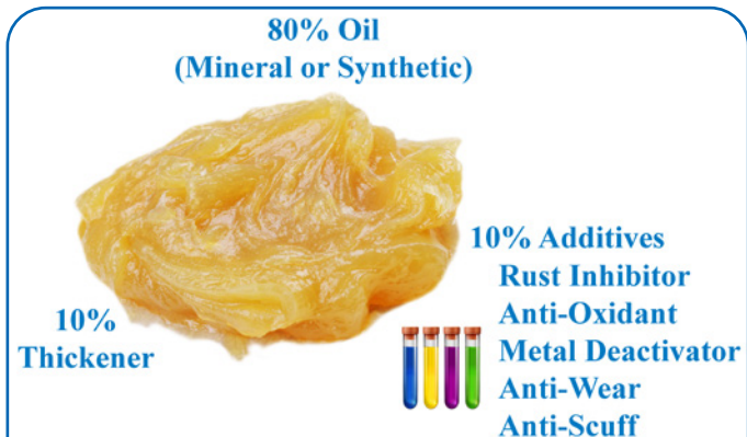
Figure 1 Diagram of grease composition (oil, thickener additive).
