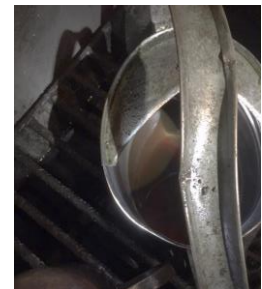
Case Study 2c – Dirty topup cans, showing grit and dirt on the handle and within the container.
