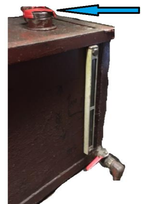
Case Study 2d – Cracked breather introducing dirt and debris into lube storage tanks.
