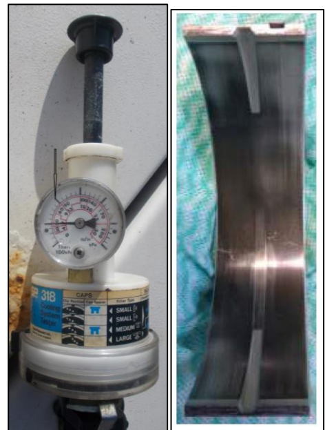
Case Study 1a – (Left) pressure of coolant showed significant drop on testing. (right) Bearing shell showed wiping from coolant
