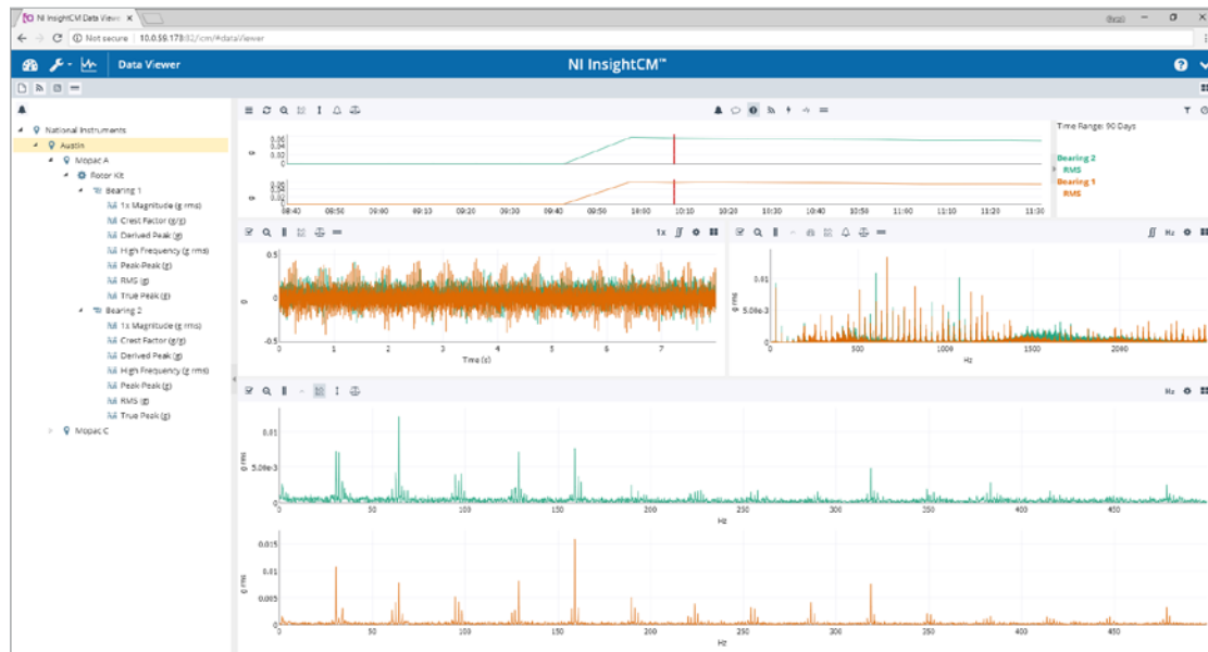
Figure 2. This vibration measurement layout shows RMS trend line, waveform, spectrum, and envelope analysis.
