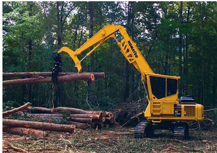
Komatsu PC290LL-11 log loader uses hydraulic power with sophisticated controls for its swing and travel drives as well as for boom, arm, and heel functions.
