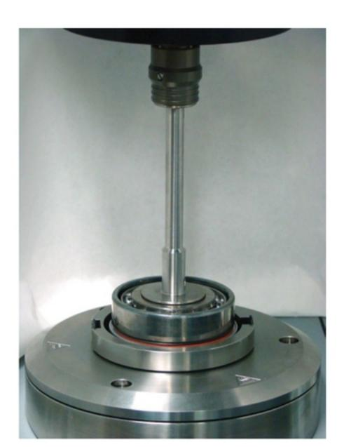
FAG FE9 bearing test set-up.
