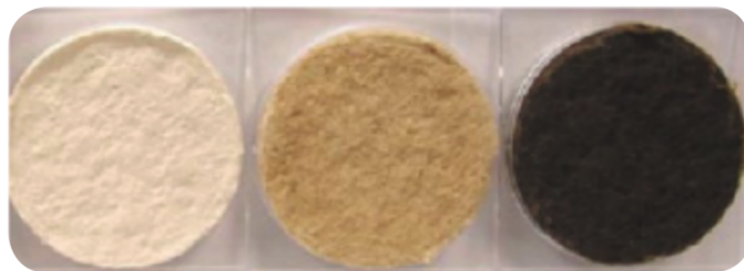
These images show a used VRF medium as received from the field (right), rinsed with hexane (center) and rinsed with toluene (left).
