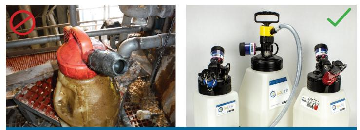
Figure 4 – the transfer container on the left has been left open and the lid has to be removed to fill it. The container on the right is completely sealed and can filled using quick connects
