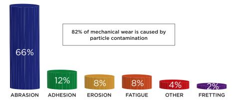
Studies show that approximately half of lost machine life is due to mechanical wear and approximately 80% of mechanical wear is caused by particle contamination in the oil. It therefore stands to reason that when particle contamination is reduced, wears rates go down and component service life goes up.
