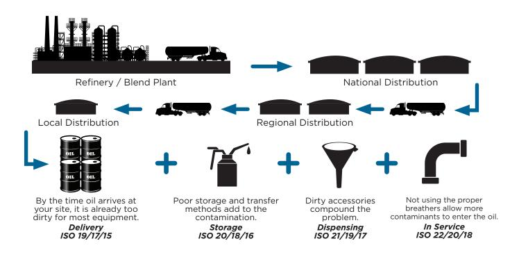
Figure 1 – Demonstrates the Lubrication System from the Refinery/Blend Plant through the dispensing into a component. From the point of delivery to each subsequent lubricant transfer, the ISO code potentially increases by at least one grade which is equivalent to doubling and in some cases tripling the amount of contaminant in the oil. As an end user, control over the lubrication system starts at the point of delivery into the plant and extends all the way through to point of use at the machine.
