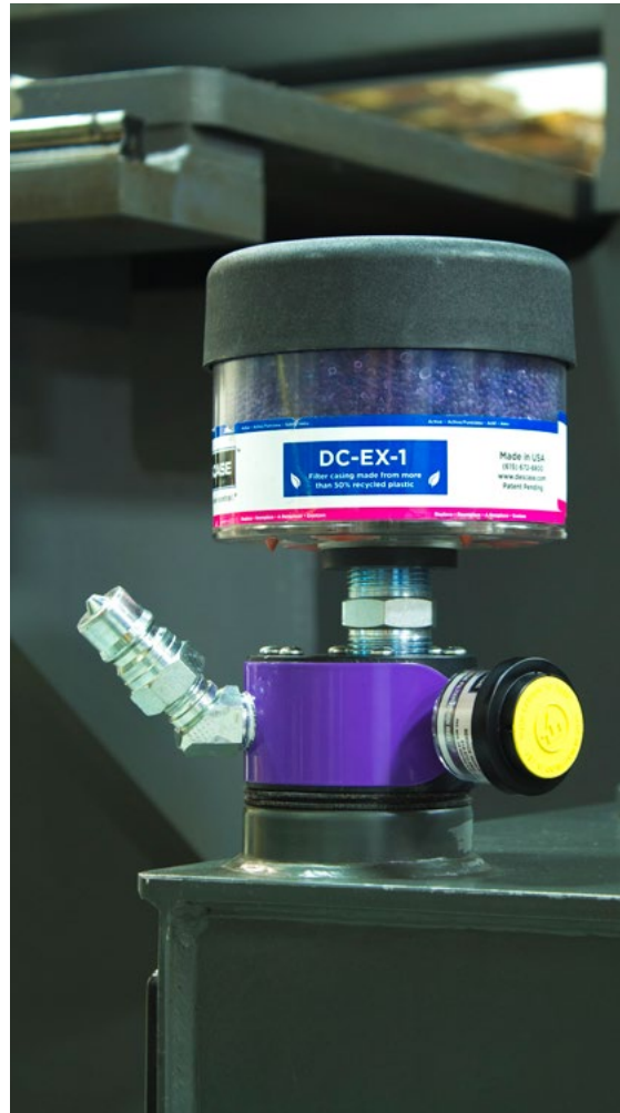
Figure 2. Desiccant breathers on tanks and reservoirs help keep water and particulates out.
