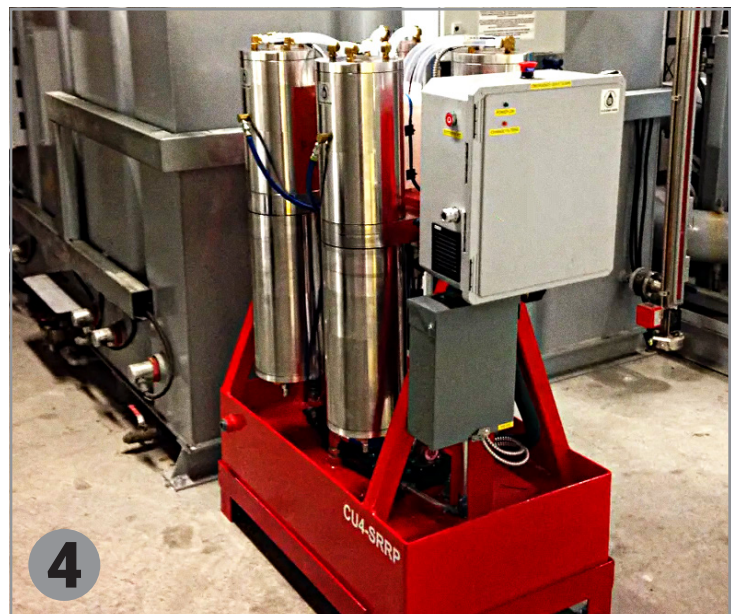
4. Four HI4 Conservor™ units mounted on a custom stationary skid. The system is installed near a large reservoir at a paper mill.
