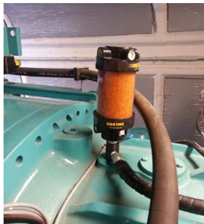
Figure 3 Do use high quality desiccant breathers
