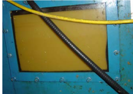
Figure 13 [Right] Sight Glass after adding Desorber
