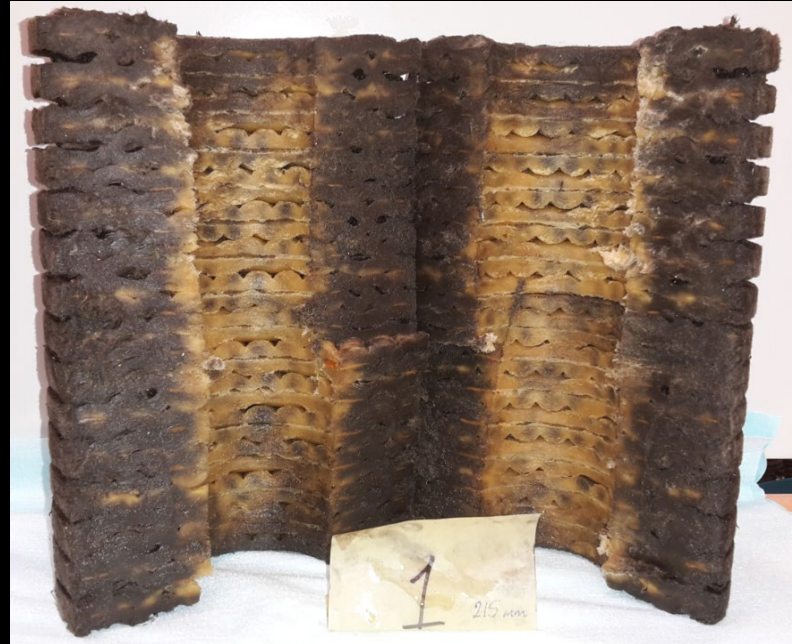
Real world results showing a cross sectional view of a used Offline Filter insert after 12 months of operation in a wind turbine gearbox. This Offline Filter insert removed 5 pounds of dirt and particles!
