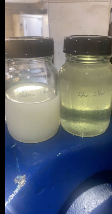
Real world results showing how effective the Offline Filter is at removing water in gear oil.
