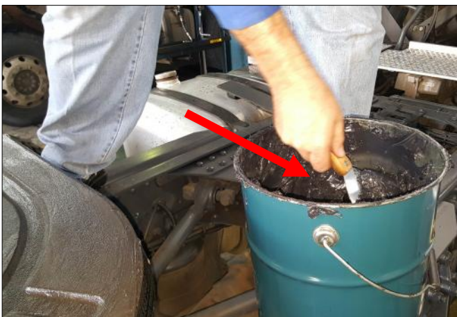
Use a scraper to scoop up fresh EP2 Graphite lubrication
