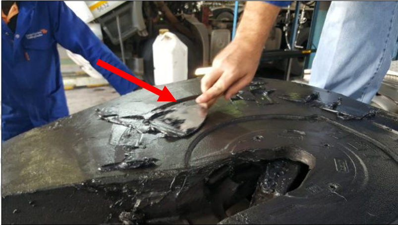
Once the entire grease groove has been filled with lubrication start spreading the grease 2mm thick over the entire raised area of the fifth wheel top plate.
