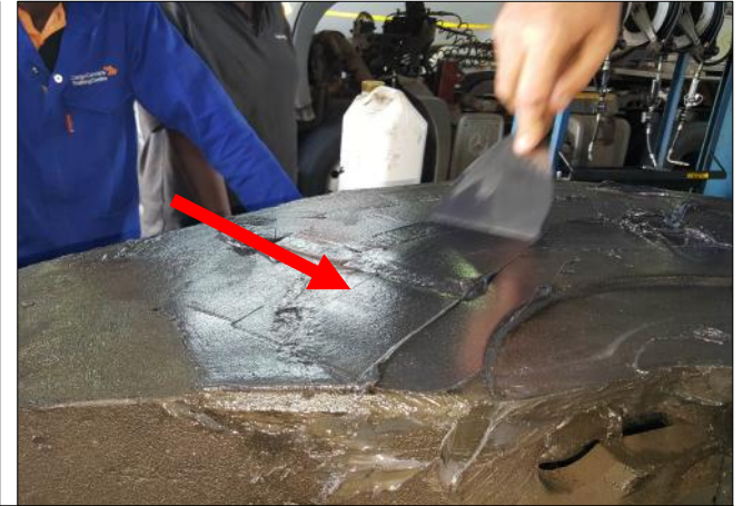
Once the entire grease groove has been filled with lubrication start spreading the grease 2mm thick over the entire raised area of the fifth wheel top plate.
