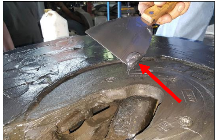
Scoop up a bit of grease on the corner of the scraper
