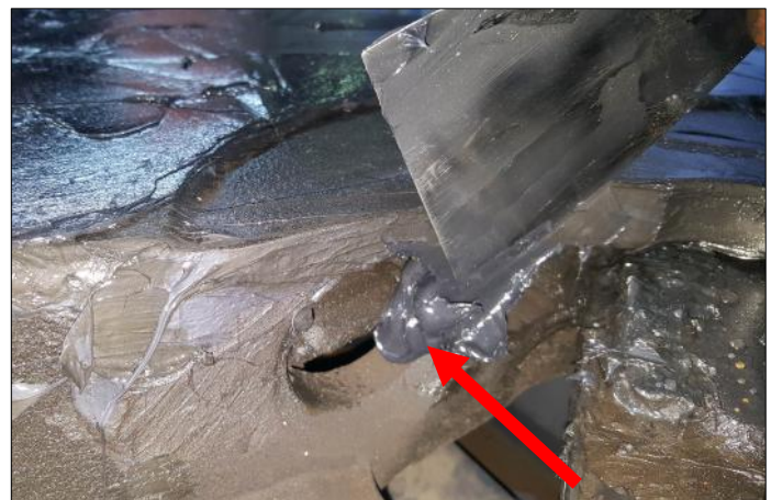
Apply a blob of grease to the inside of the wearing ring and in the hole on the left where the lockjaw will scoop it up as it closes around the kingpin when hitching.
