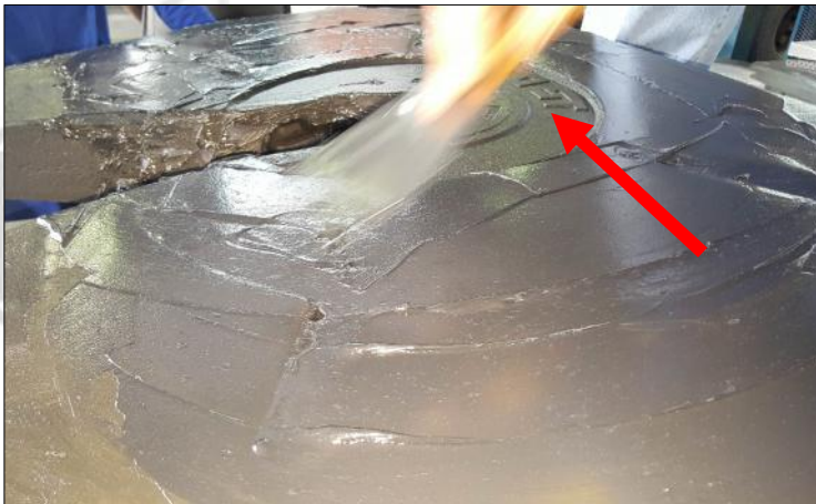
Keep the central lower area of the fifth wheel top plate clean.
