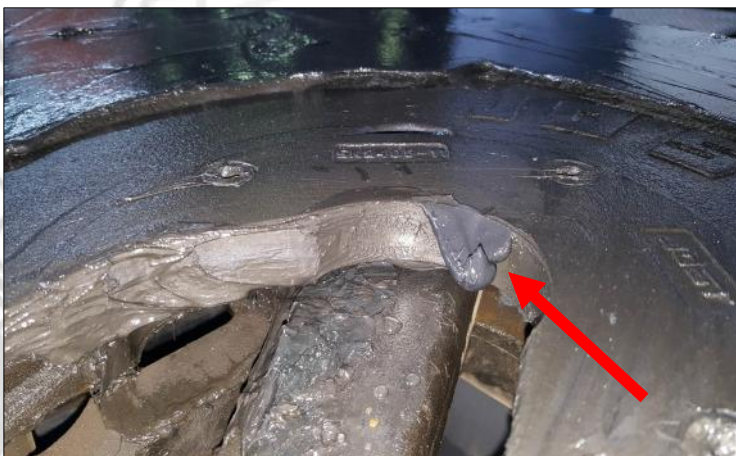
Apply a blob of grease to the inside of the wearing ring and in the hole on the left where the lockjaw will scoop it up as it closes around the kingpin when hitching.
