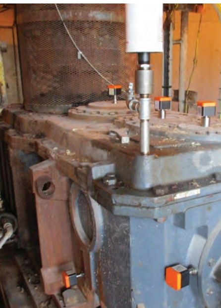
An I-DNA installation on a gearbox
