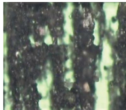
Figure 7 | Black oxides, lubricant starvation.
