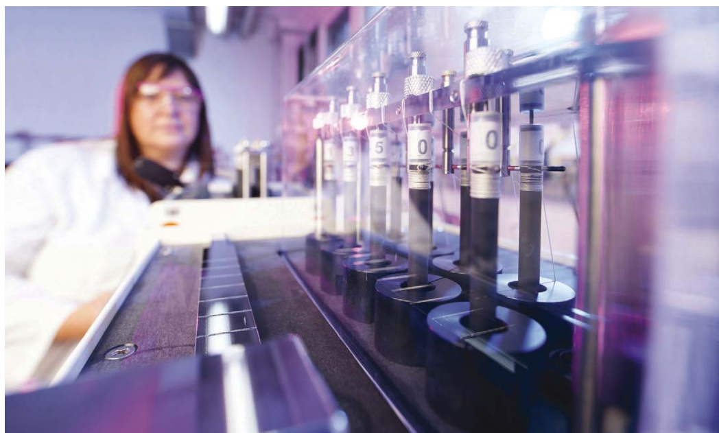
An MRV test is run at Evonik’s lab in Darmstadt, Germany. (Photo: Evonik)
