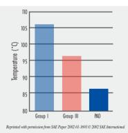
This lower operating temperature, along with the superior oxidative stability of PAO-based lubes can aid in increasing the service life of the lubricant and decrease the generation of corrosive agents that can damage your lubricated system.
