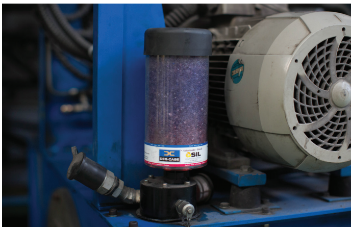
BREATHER ADSORBING EXTERNAL MOISTURE
