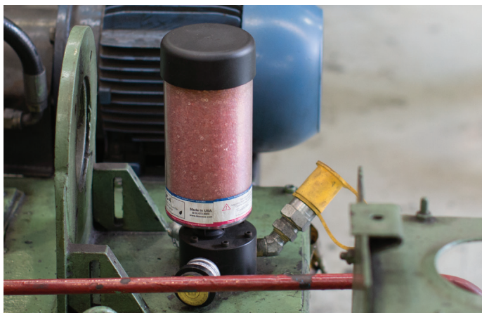
FULLY SATURATED AND SPENT BREATHER
