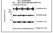
Once spalling occurs, it accelerates very quickly. The contact area becomes much larger, and the pressure becomes more volatile. As a result, it is difficult for the lubricant wedge to maintain its shape, and surfaces can no longer remain separate. The spalling then accelerates quite quickly.
