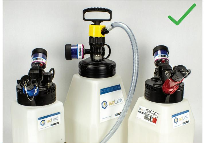
Figure 4 - the transfer container on the left has been left open and the lid has to be removed to fill it. The container on the right is completely sealed and can be filled using quick connects
