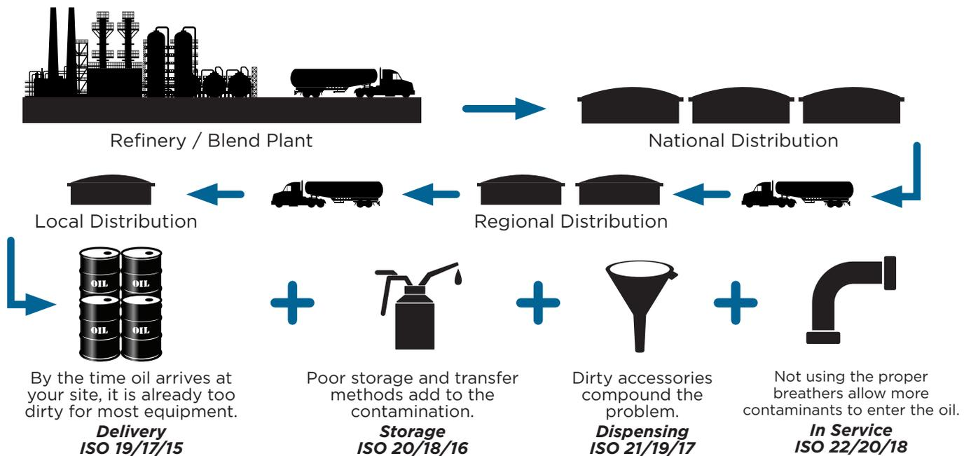
Figure 1 - Demonstrates the Lubrication System from the Refinery/Blend Plant through the dispensing into a component. From the point of delivery to each subsequent lubricant transfer, the ISO code potentially increases by at least one grade which is equivalent to doubling and in some cases tripling the amount of contaminant in the oil. As an end user, control over the lubrication system starts at the point of delivery into the plant and extends all the way through to point of use at the machine.
