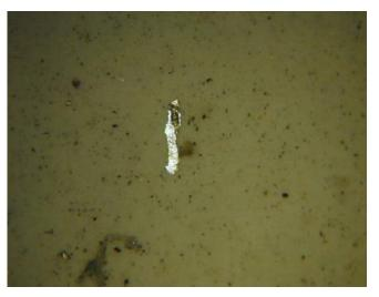
160 micron ferrous sliding wear particle
