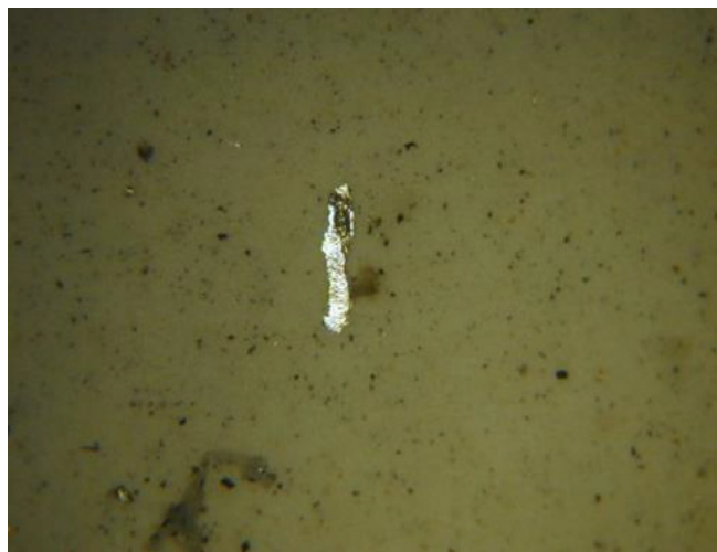
160 micron ferrous sliding wear particle
