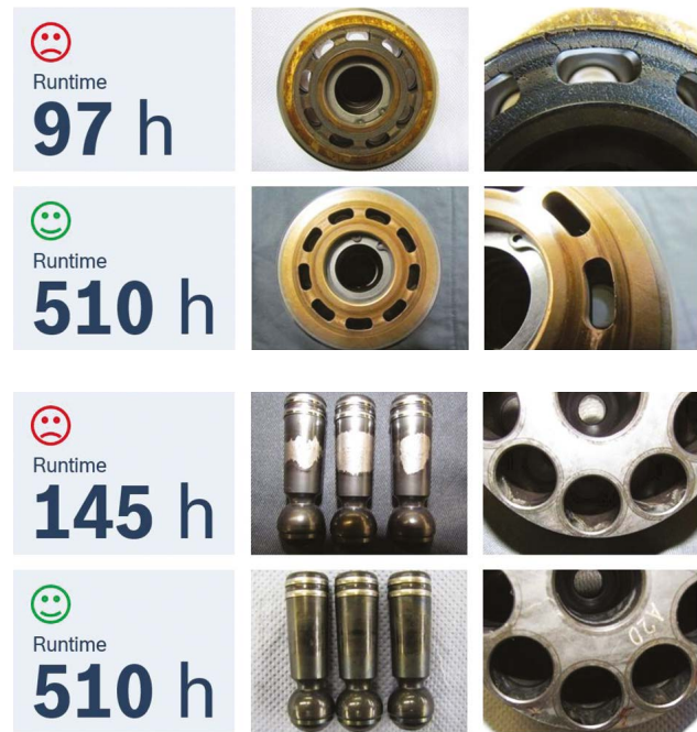
Figure 6a+b. On the one hand, Bosch Rexroth tests show fluids that have led to significant damage after fewer than 100 operating hours. Other hydraulic fluids cause no wear whatsoever after 510 hours. (Copyright: Bosch Rexroth AG)².
