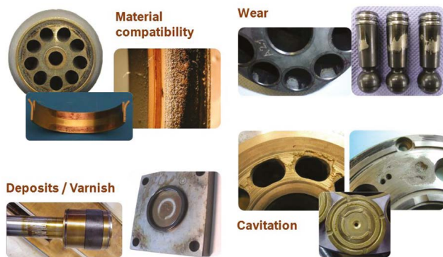
Figure 2. Causes of failure due to fluid (Copyright: Bosch Rexroth AG)
