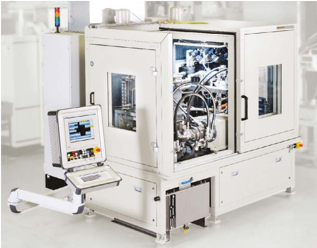
Figure 7. Abb. 7: If desired, Bosch Rexroth also offers an RFT-APU-CL fluid test bench that the manufacturers of lubricants and additives can use in test laboratories for their own development work, for example. (Copyright: Bosch Rexroth AG)
